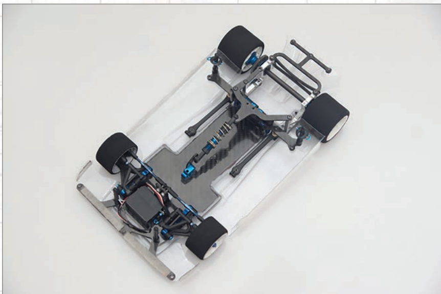
The Vectorworks Hornet with custom carbon fiber chassis and Lexan diffuser panels.
