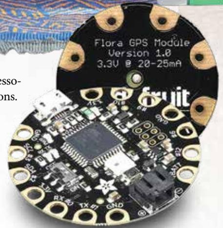
The Adafruit Flora has a circular shape with large input and output holes that make it easy to add to a soft good.
