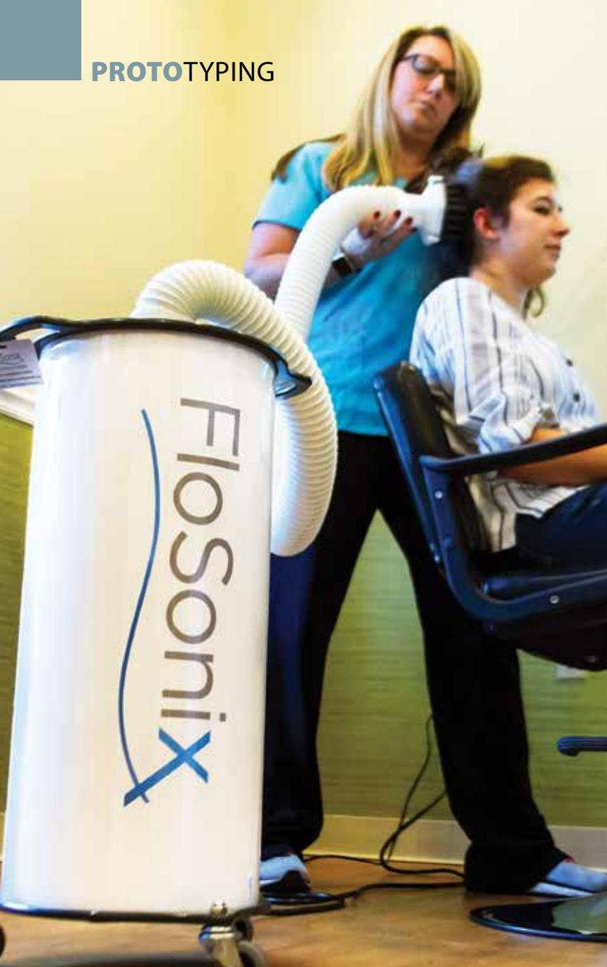
The FloSonix lice treatment device was built on the Particle platform, to allow the Eventys Partners team to monitor key performance parameters and update the device firmware.
