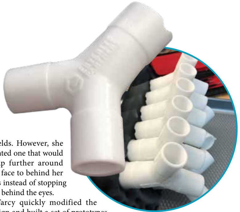
A Y-splitter enables the use of one ventilator for multiple patients.
