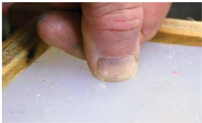
You can test the durometer of silicone rubber with a thumbnail.
