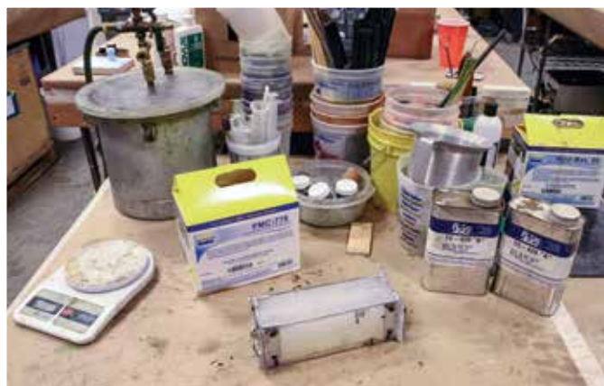
The Enventys molding station shows a silicone mold, digital scale, vacuum chamber and mold kits.
