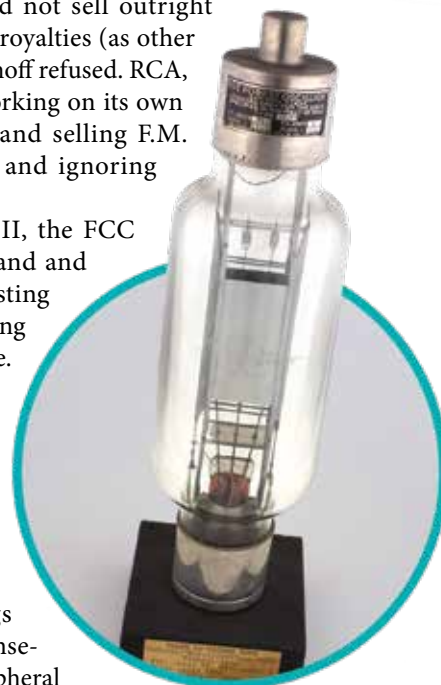
Lee de Forest's Audion (triode) vacuum tube was the first practical amplification device. Pictured is his Type 2Q15 triode, circa 1921. Although he had more than 300 patented inventions, de Forest was often involved in litigation regarding his business ventures.
