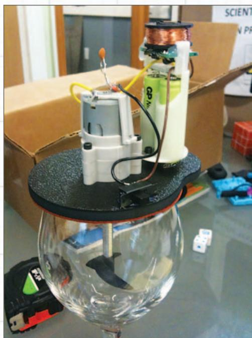
Early Wine Shark prototypes were made from inexpensive raw materials and mechanical components harvested from an off-the-shelf immersion blender.
